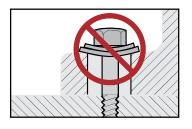
mended cap screw or thread is specified on the product page of this catalog. Sometimes the mounting hardware is included with the component. Always use supplied hardware.
