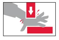
Do not require the operator to hold the workpiece in position during the clamping operation. Make sure that the workpiece is self-supporting and self-locating so that operator hands are out of
